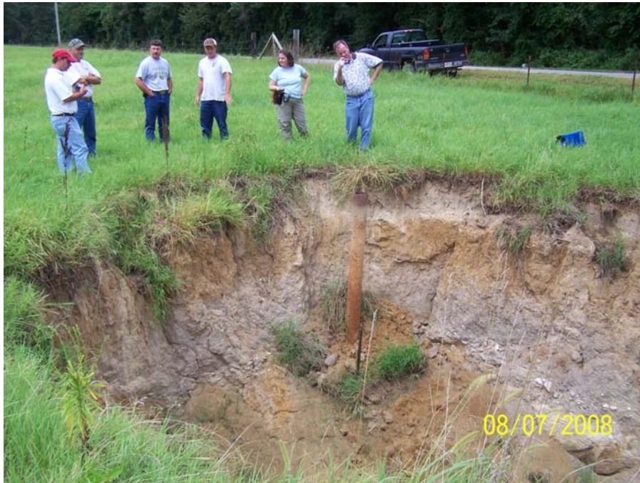
Sinkhole formed around abandoned well bore, view looking northwest. Note soil horizon of ~6 feet and regolith below soil. Looking northwest.
