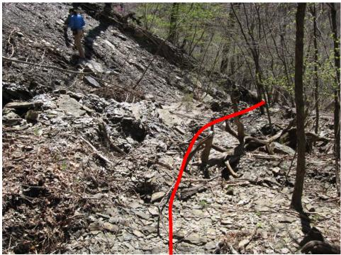
This photo displays the southern edge of the slide with the red line illustrating the path water flowed from below small bluff line.
