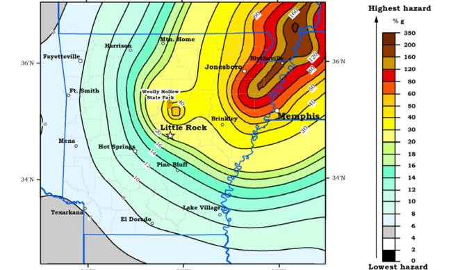
Seismic Hazard is expressed as Peak Ground Acceleration (PGA) on firm rock, in percent g, expected to be exceeded in a 50 year interval with a probability of two percent Source: National Seismic Hazard Mapping Project (2016)
