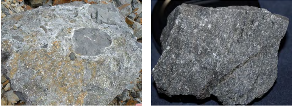
Figure 5. Tuff containing shale clasts (left) and fine-grained tuff containing white feldspar fragments (right).
