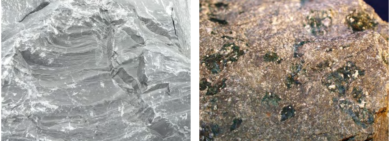
Figure 18. Fine-grained gray tuff displaying small scale cross-bedding (left). Large (1-2cm) green lapilli in a fine-grained matrix (right).
