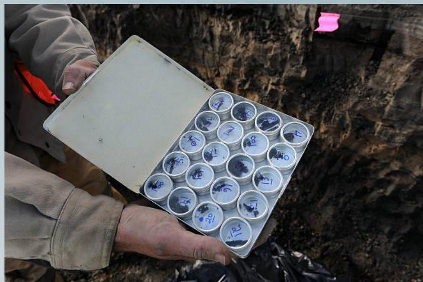
**Sand samples for grain size analysis. Laser Diffraction technique.**
