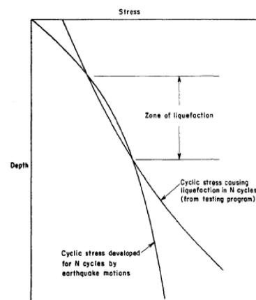
Figure 1. Method of evaluating liquefiable zone
