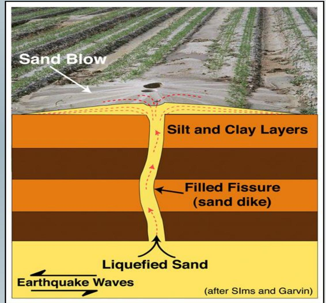
Schematic showing a sand dike and sand blow (from USGS).
