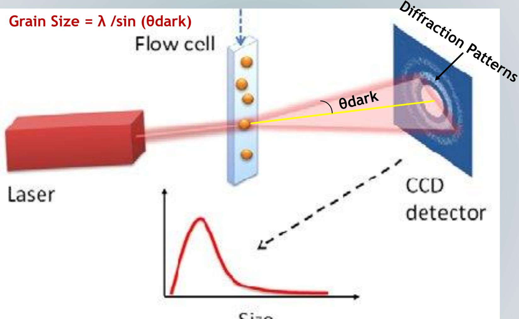
Principles of laser diffraction measurements (Hyll, 2015).
