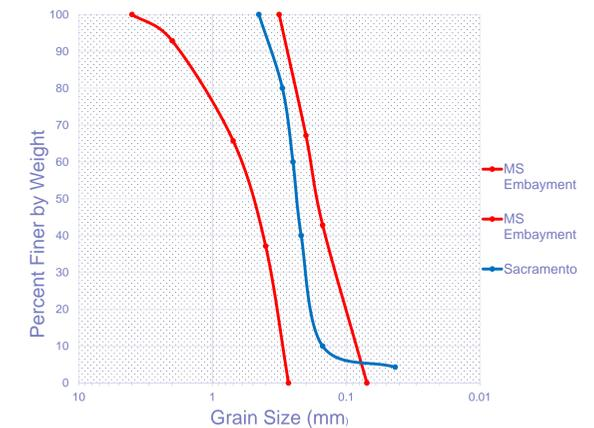
Figure 3. Comparison of the grain size distribution of Sacramento River sand and MS Embayment sand
