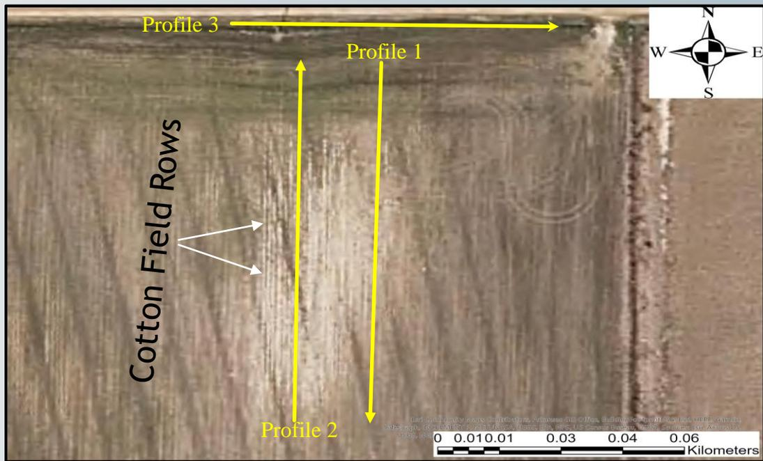
GIS Imagery showing the location of GPR profiles (yellow solid lines) collected on Site-1 (DBSE1). The light-colored soils indicate the location of the potential sand blow.
