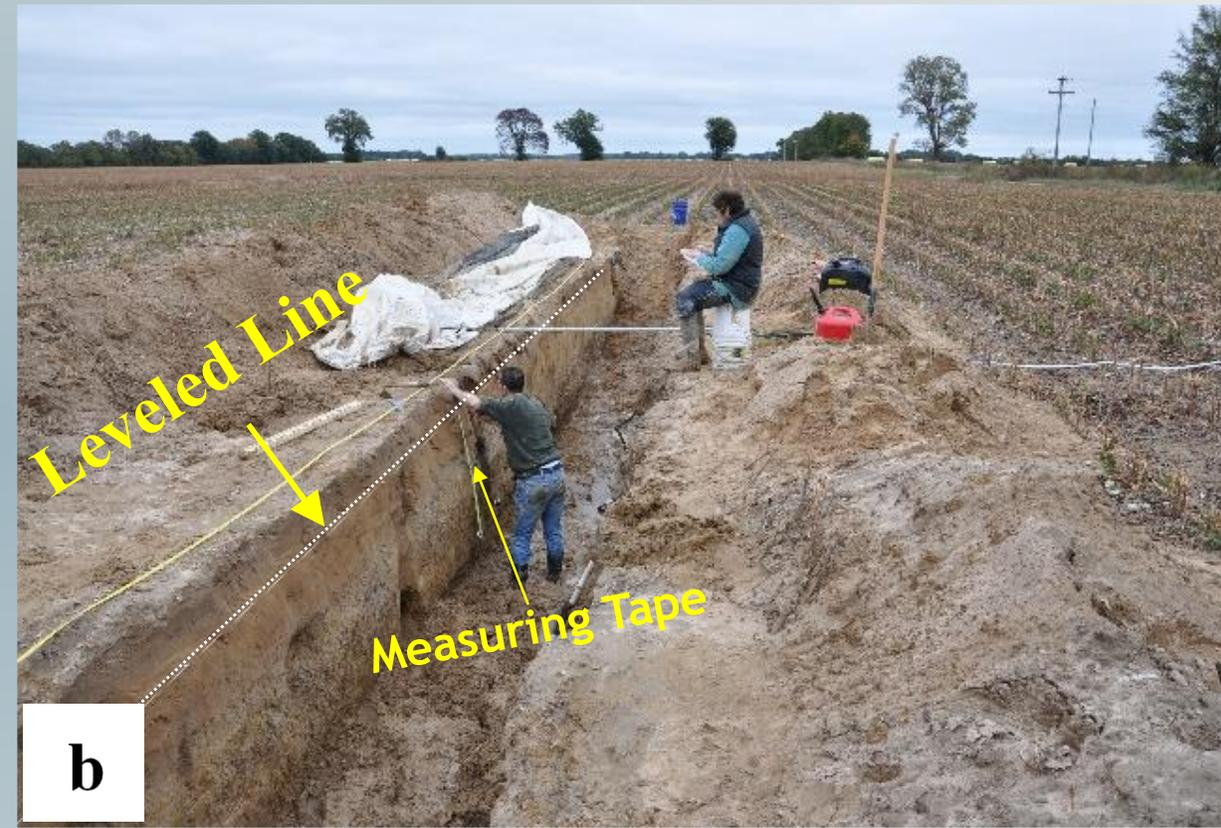
Photographs showing the logging work at DBNW3: a) Logging at the northern trench (DBNW3N), and b) Logging at the southern trench (DBNW3S).
