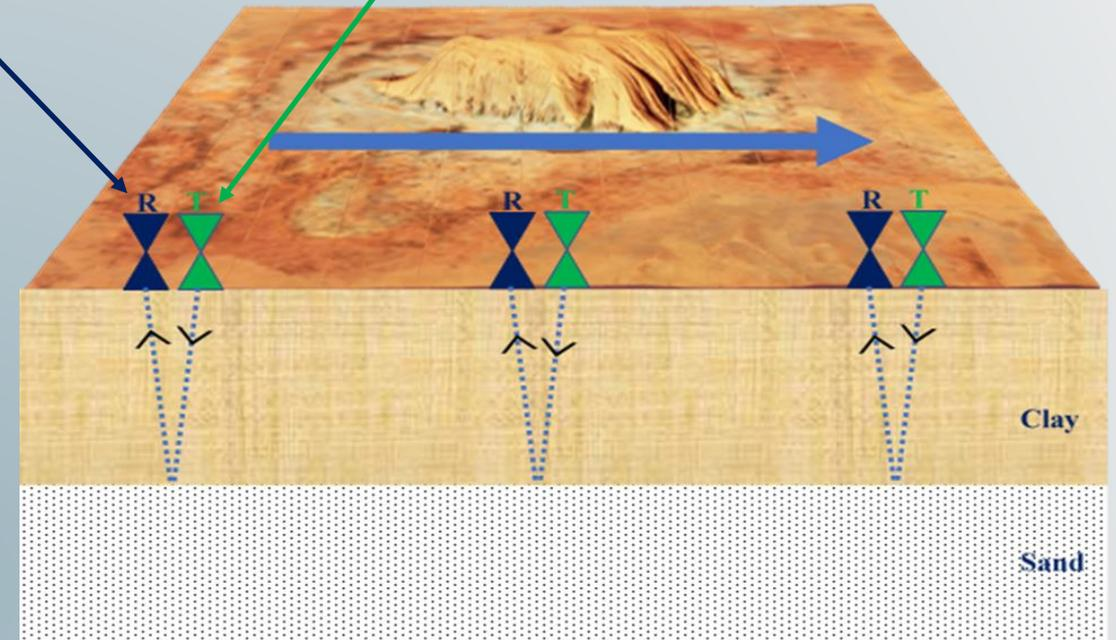
Schematic image showing reflection GPR mode.
