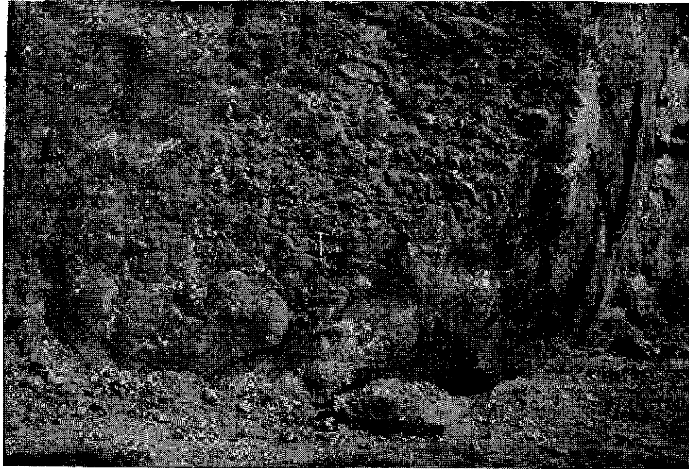
Figure 4. — Novaculite breccia at the top of the Upper Division of the Arkansas Novaculite at the Dempsey Cogburn mine. The face on the right is a cross fault showing novaculite below the breccia zone.
