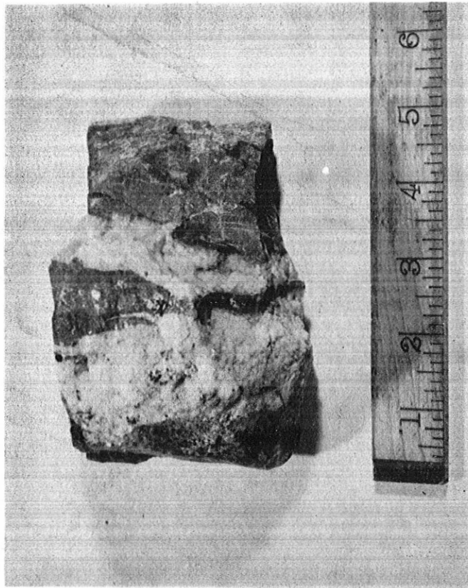
Photograph of barium, strontium and calcium carbonate veins (white) cutting dense barite (black). Foot wall ramp, Baroid pit, Magnet Cove district.
