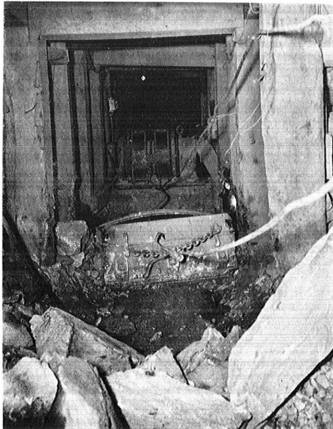
Photograph showing operations in a scraper drift, Magcobar underground mine, Magnet Cove district. (Photographer, Fred A. Burnett)
