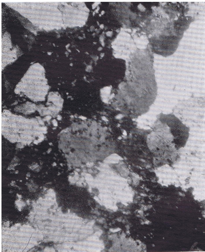
PLATE 18. Microphotograph. Same as Plate 17 but with crossed nicols. Shows quartz anhedral with smaller quartz crystals. Attention is called to the very irregular outline of the grains. All quartz is of the same generation.
