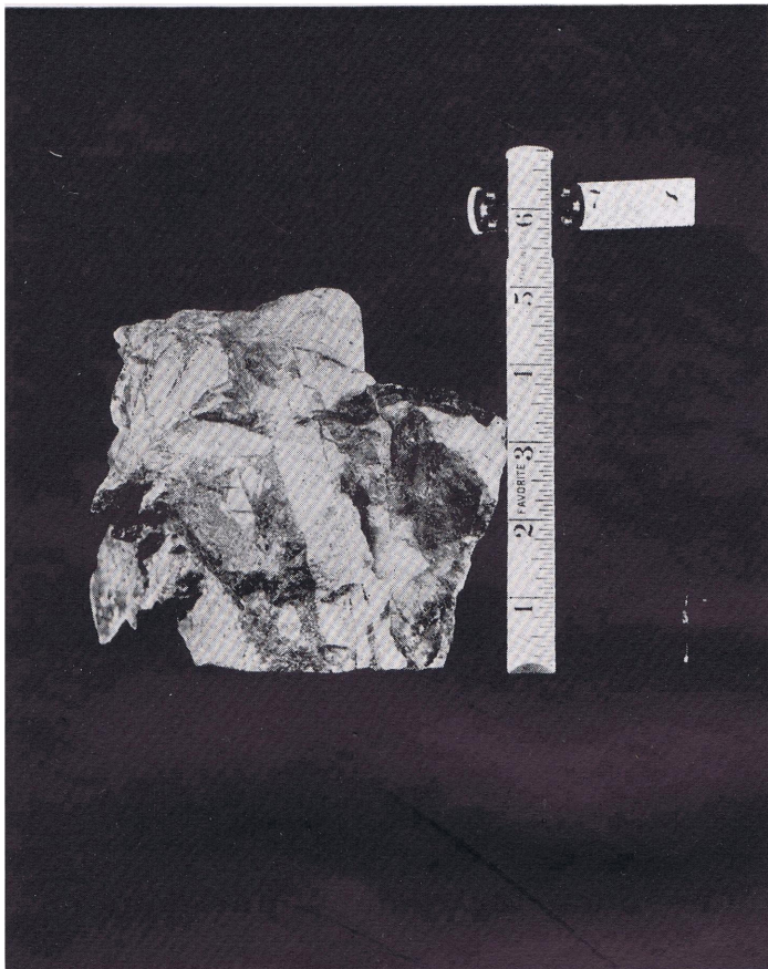
PLATE 8. Specimen of cinnabar and sandstone breccia. Darker material is cinnabar. From the Parker property, sec. 11, T. 7 S., R. 26 W.
