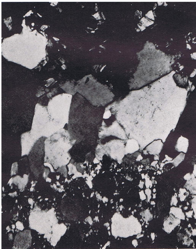
PLATE 12. Microphotograph. Same as Plate 11 but with crossed nicols. The sharp boundary between the vein quartz and dickite gouge should be particularly noticed.
