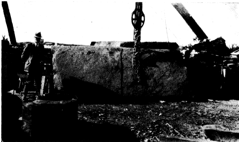
B. A block of black marble, 10'x4'x8", from the Fayetteville formation, ready for shipment at the Batesville Black Marble Company's yard, Batesville.
