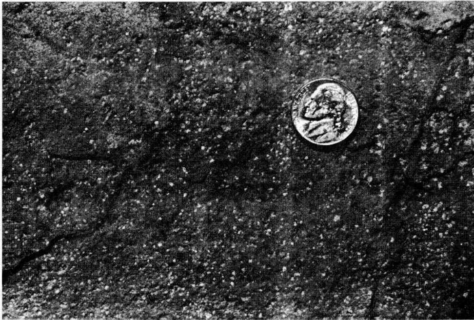
Figure 12b – The rock is gray-green, tough, fine-grained, and often contains sedimentary clasts. The principal mineral is olivine, largely altered to serpentine, with detrital quartz being common. Bedding is evident in some fragments.
