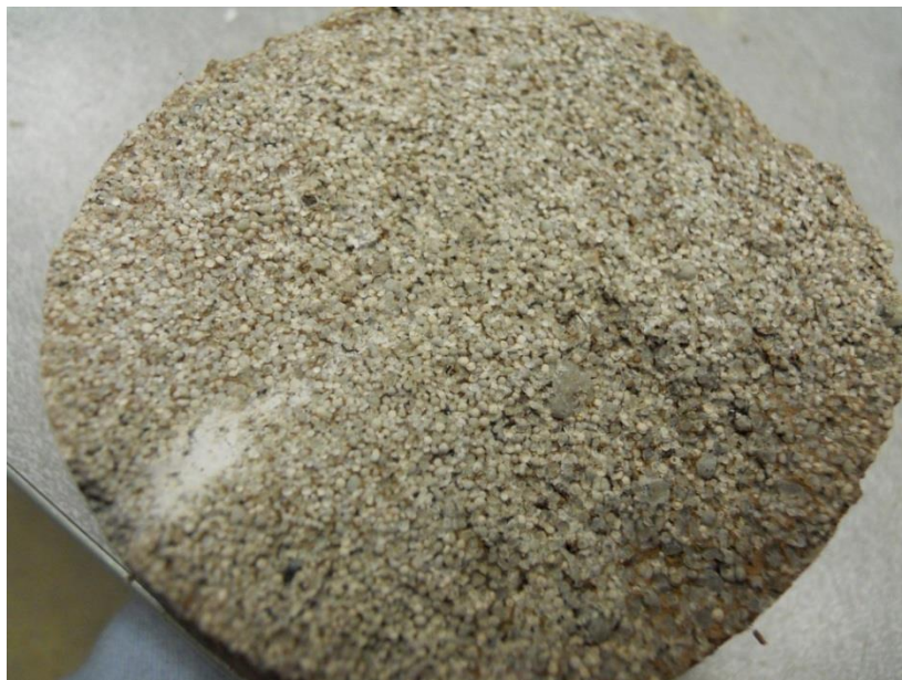
Figure 7. Oolitic grainstone of the upper Smackover Formation. Permit number 26489, western Union County. Core diameter is 8.9 cm (3.5 in.).
