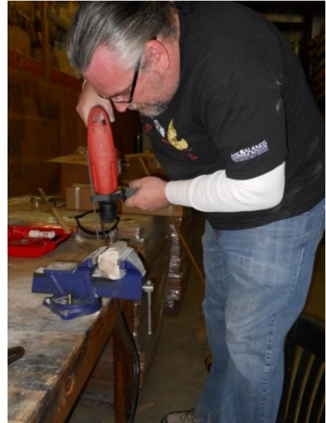
Figure 6. Hilti rotary hammer used for core sample drilling.
