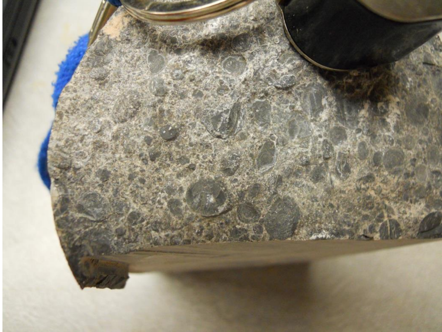
Figure 8. Oolitic to pisolitic crystalline limestone of the upper Smackover Formation. Permit number 30929, southwestern Columbia County.
