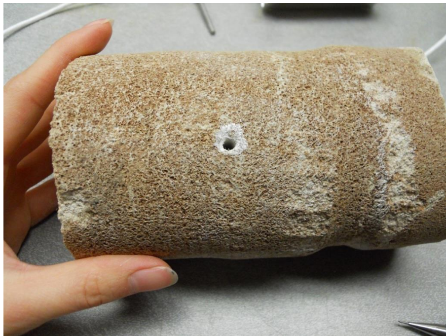
Figure 9. Oolitic grainstone exhibiting oomoldic porosity. Permit number 28301, southeastern Nevada County. Sample length approximately 20 cm (8 in). Probe hole in center of core.
