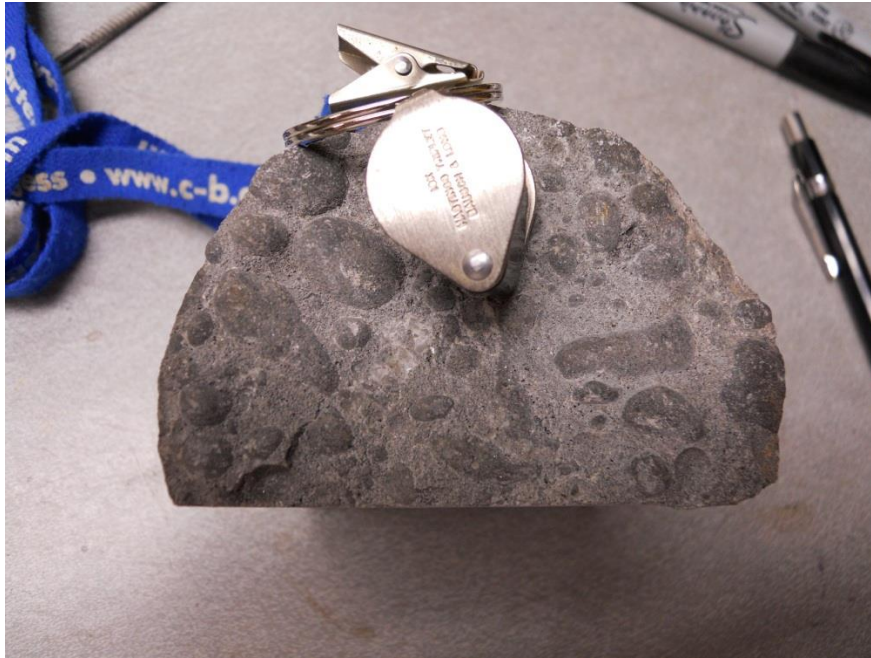
3. Possible allochems within crystalline limestone sample of upper Smackover Formation. Permit number 30929, southwestern Columbia County. Core diameter approximately 8.9 cm (3.5 in.). Hand lens for scale.
