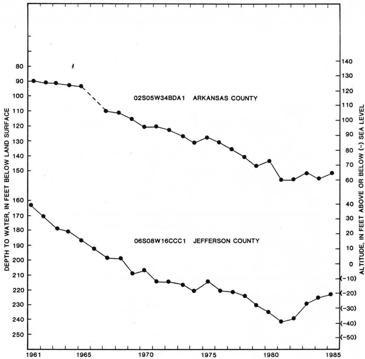
Figure 2. sheet 1 of 2.--Water-level hydrographs for selected wells completed in the Sparta Sand.
