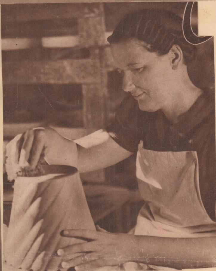
WHEN THE POTTER IS DONE WITH THE PIECE, there is yet needed an all-over smoothing with a wet sponge. That is what the "finisher" here is doing.
