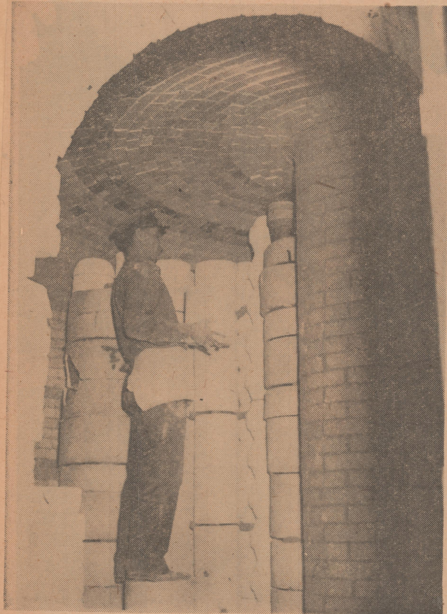
Pieces to be fired to 2,000 degrees by gradual heating, followed by gradual cooling, are being placed in the kiln. Exact temperature control, plus skill and knowledge, make this ware uniform to conform to rigid government specifications.
