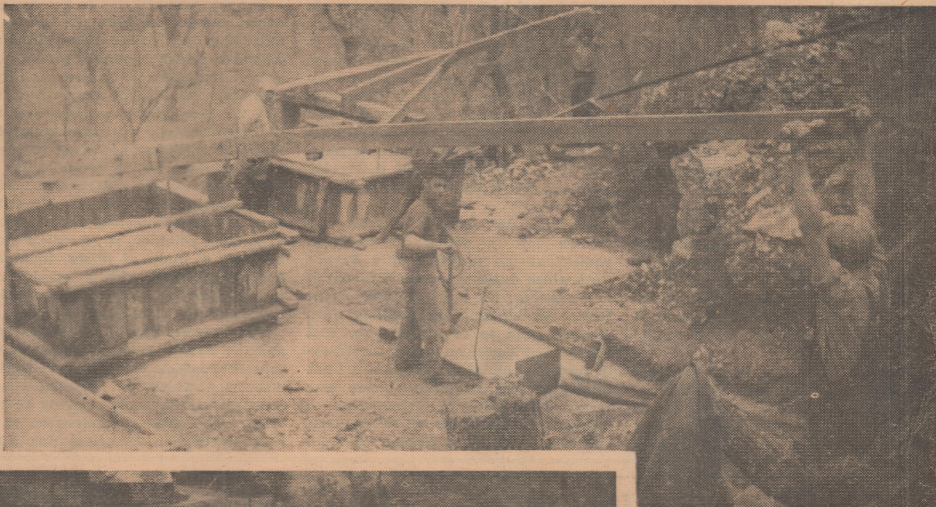
Workers in a Boone county mine are hand jiggling ore in the picture above. At the left is a scene at the Monte Cristo Concentrating Plant, Rush Creek Camp, Marion county.
