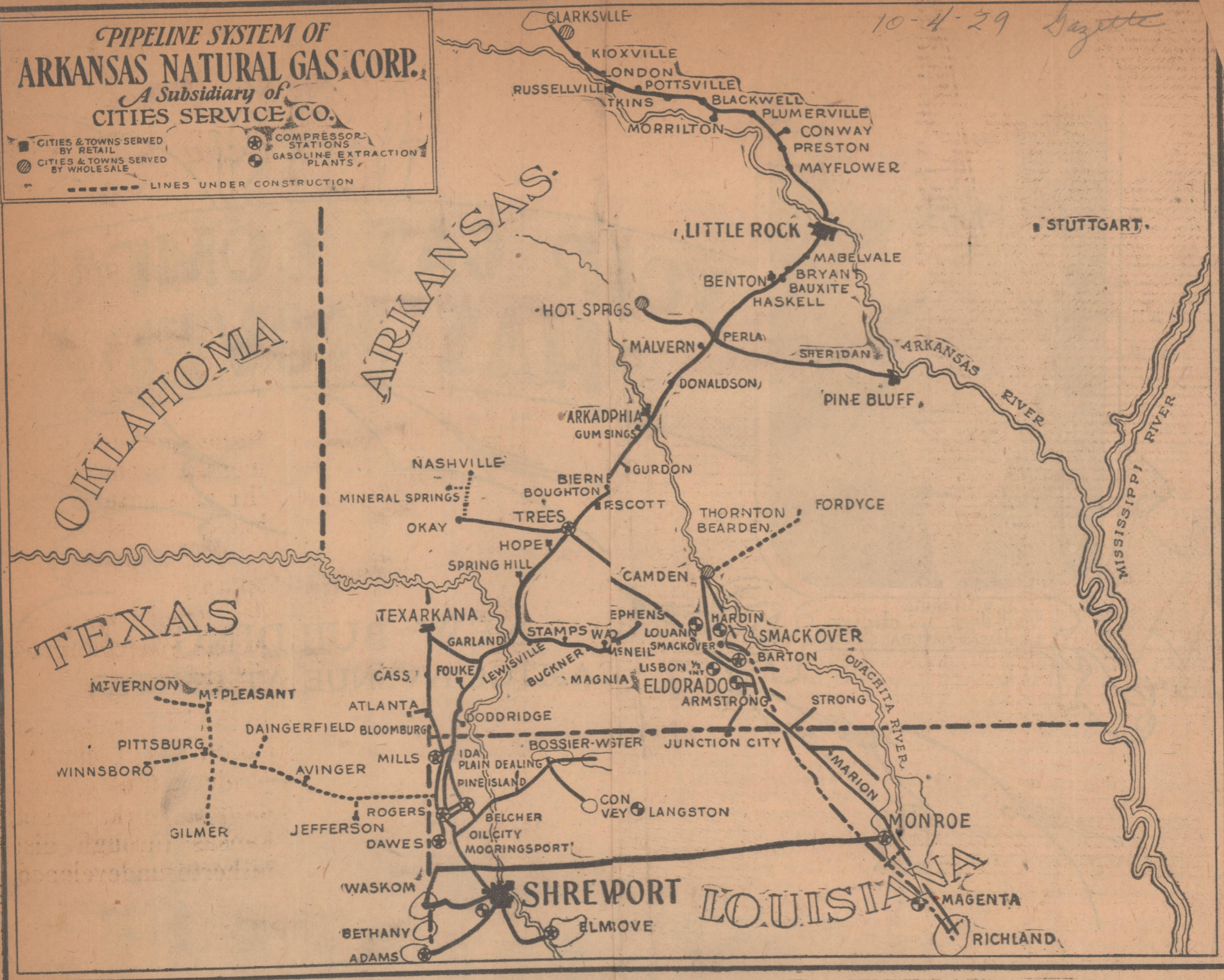
Above is the latest map of the Arkansas Natural Gas Corporation's pipe lines, gasolants and compressor stations. It shows the 20 inch pipe line from Monroe and Richland, the second largest gas field in the world, to the company's main system near Shreveport. It also pictures the beginning of a new line into East Texas to serve eight cities. It gives view of the projected line to Nashville, Ark., through Mineral Springs. It shows new Muncie Compressor Station, the largest in the world, near Monroe, and the Barton Compressor Station El Dorado. The map demonstrates the inter-connected system from four major fields, thus assuring uninterrupted supply of gas for all purposes at all times.
